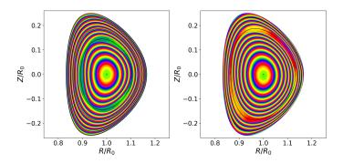
Nevertheless, when perturbed electron temperature added to equilibrium temperature, result is appropriate helical flat-spot at NTM rational surface.
