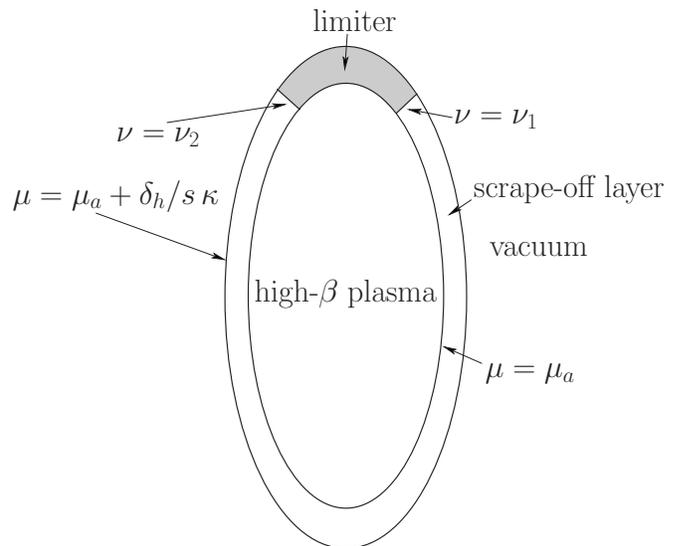
FIG. 1. Schematic diagram showing the poloidal cross section of a high- $\beta$  plasma surrounded by an axisymmetric halo consisting of a low- $\beta$  scrape-off layer and a rigid conducting limiter.
