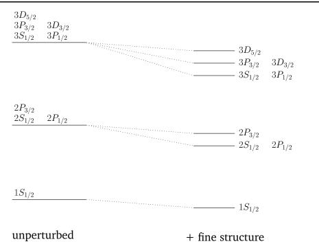
Figure 12.1: Effect of the fine structure energy-shift on the n = 1, 2 and 3 states of a hydrogen atom. Not to scale.
