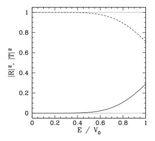
Figure 5.3: Transmission (solid-curve) and reflection (dashed-curve) probabilities for a square potential barrier of width  $a = 0.5 \lambda$ , where  $\lambda$  is the free-space de Broglie wavelength, as a function of the ratio of the energy, E, of the incoming particle to the height, V<sub>0</sub>, of the barrier.
