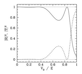
Figure 5.1: Transmission (solid-curve) and reflection (dashed-curve) probabilities for a square potential barrier of width  $a = 1.25 \lambda$ , where  $\lambda$  is the free-space de Broglie wavelength, as a function of the ratio of the height of the barrier, V<sub>0</sub>, to the energy, E, of the incident particle.
