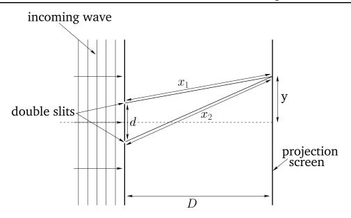
Figure 3.5: Classical double-slit interference of light.
