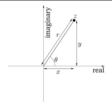
Figure 3.3: Representation of a complex number as a point in a plane.
