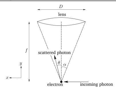
Figure 3.8: Heisenberg's microscope.
