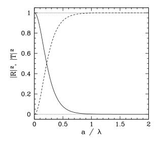
Figure 5.4: Transmission (solid-curve) and reflection (dashed-curve) probabilities for a particle of energy E incident on a square potential barrier of height  $V_0 = (4/3)$  E, as a function of the ratio of the width of the barrier, a, to the free-space de Broglie wavelength,  $\lambda$ .
