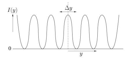
Figure 3.6: Classical double-slit interference pattern.
