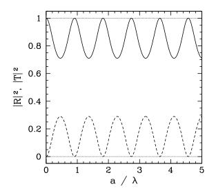
Figure 5.2: Transmission (solid-curve) and reflection (dashed-curve) probabilities for a particle of energy E incident on a square potential barrier of height  $V_0 = 0.75$  E, as a function of the ratio of the width of the barrier, a, to the free-space de Broglie wavelength,  $\lambda$ .
