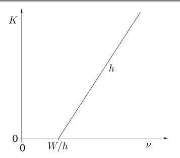
Figure 3.4: Variation of the kinetic energy K of photoelectrons with the wave-frequency v.
