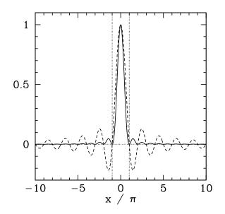
Figure 13.1: The functions sinc(x) (dashed curve) and  $sinc^2(x)$  (solid curve). The vertical dotted lines denote the region  $|x| \le \pi$ .
