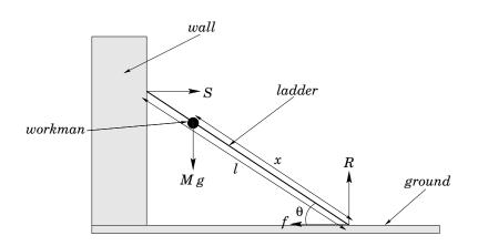
Figure 93: A ladder leaning against a vertical wall.
