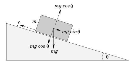
Figure 33: Block sliding down a rough slope
