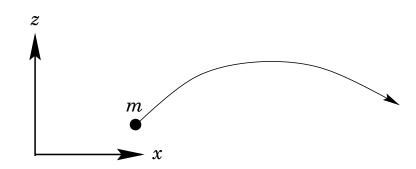
Figure 35: Coordinate system for 2-dimensional motion under gravity
