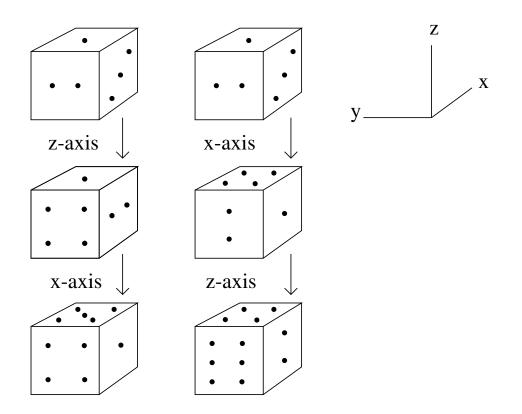
Figure 69: *The addition of rotation is non-commutative*.
