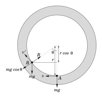
Figure 65: Motion on the inside of a vertical hoop.
