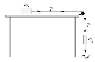
Figure 30: Block sliding over a smooth table, pulled by a second block
