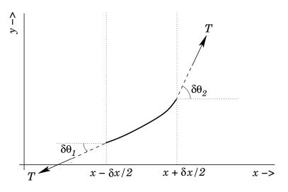
Figure 108: Forces acting on a segment of a stretched string.
