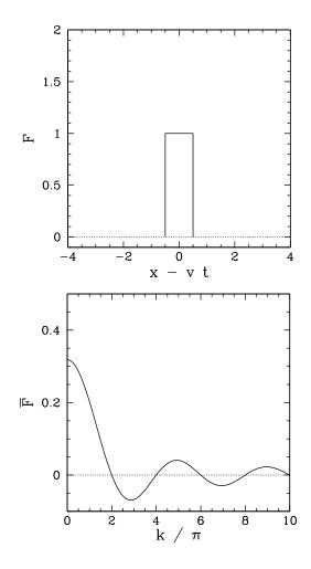
Figure 111: A propagating wave-pulse, F(x - v t), and its associated Fourier spectrum,  $\overline{F}(k)$ .
