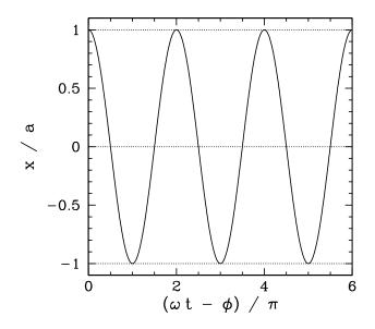
Figure 95: Simple harmonic motion.
