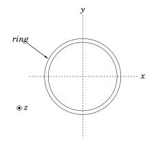
Figure 77: The moment of inertia of a ring about a coplanar symmetric axis.
