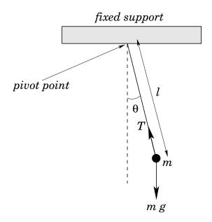
Figure 97: A simple pendulum.
