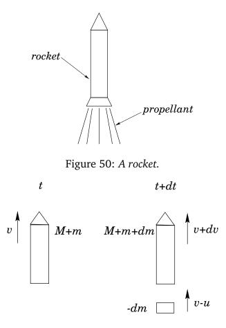
Figure 51: Derivation of the rocket equation.
