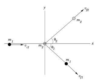
Figure 55: A collision in 2-dimensions.
