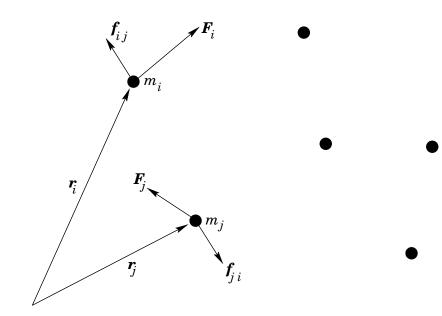
Figure 48: A 3-dimensional dynamical system consisting of many point mass objects.
