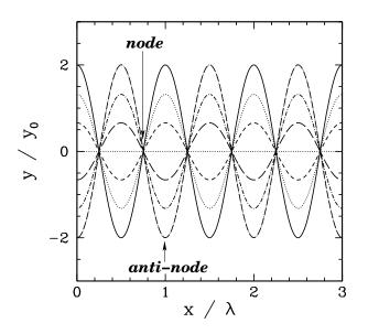
Figure 113: A standing wave. The various curves show the wave displacement at different times.
