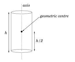
Figure 73: Locating the geometric centre of a right cylinder.
