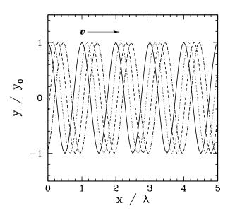
Figure 109: A sinusoidal wave propagating down the x-axis. The solid, dotted, dashed, and dotdashed curves show the wave displacement at four successive and equally spaced times.
