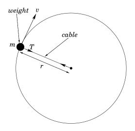
Figure 59: Weight on the end of a cable.
