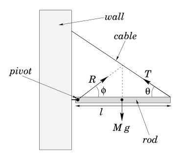
Figure 92: A rod suspended by a fixed pivot and a cable.
