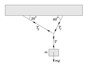
Figure 27: Block suspended by three strings
