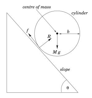
Figure 84: A cylinder rolling down a rough incline.
