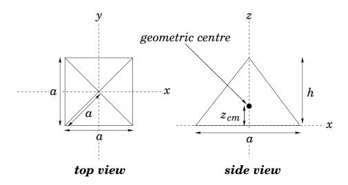
Figure 74: Locating the geometric centre of a regular square-sided pyramid.
