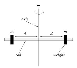
Figure 88: Two movable weights on a rotating rod.
