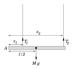
Figure 91: A horizontal rod suspended by two vertical cables.
