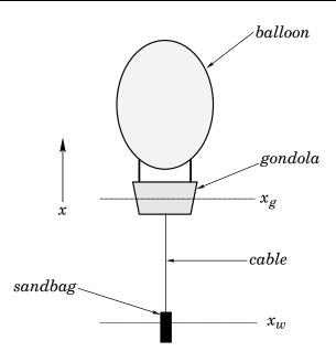
Figure 46: An example two-component system
