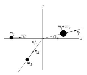
Figure 56: A totally inelastic collision in 2-dimensions.
