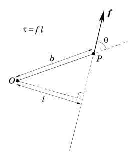
Figure 80: Definition of the length of the level arm, l.
