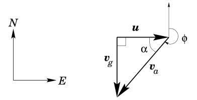
ity  $\mathbf{v}_g$  relative to the ground is the vector sum of its velocity  $\mathbf{v}_a$  relative to the air, and the velocity  $\mathbf{u}$  of the wind relative to the ground. We know that  $\mathbf{u}$  is directed due East, and we require  $\mathbf{v}_g$  to be directed due South. We also know that
