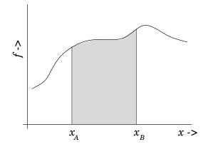
Figure 39: Work performed by a 1-dimensional force
