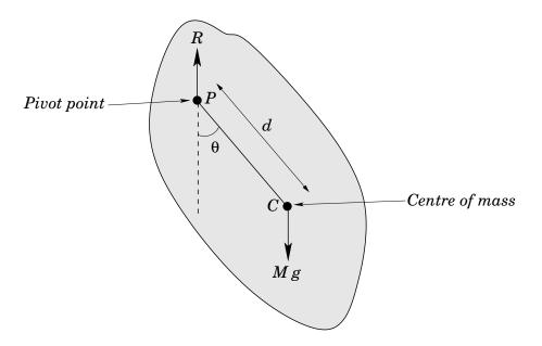
Figure 98: A compound pendulum.
