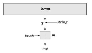
Figure 26: Block suspended by a string
