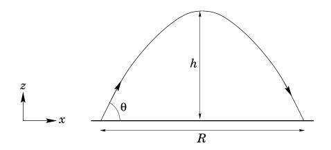
Figure 17: The parabolic trajectory of a projectile
