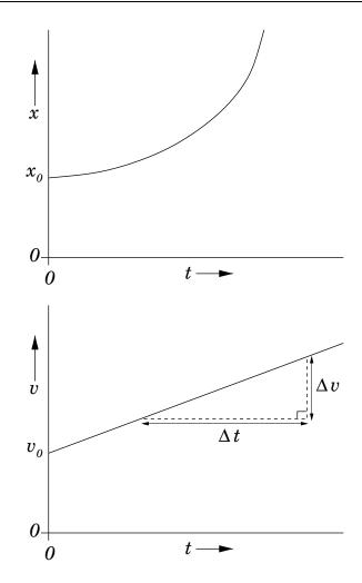
Figure 8: Graphs of displacement versus time and velocity versus time for a body moving with constant acceleration
