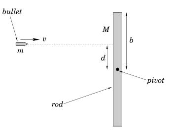
Figure 89: A bullet strikes a pivoted rod.
