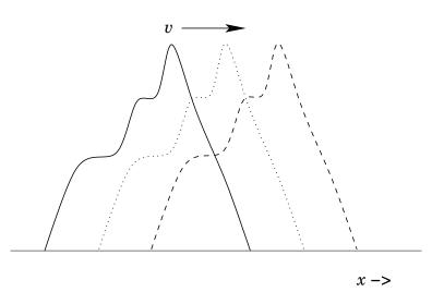
Figure 110: A wave-pulse propagating down the x-axis. The solid, dotted, and dashed curves show the wave displacement at three successive and equally spaced times.
