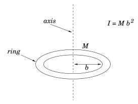
Figure 75: The moment of inertia of a ring about a perpendicular symmetric axis.
