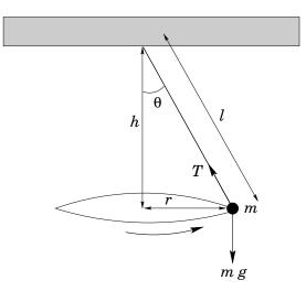
Figure 60: A conical pendulum.
