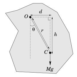
Figure 90: A laminar object pivoting about a fixed point in a gravitational field.
