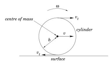
Figure 83: A cylinder rolling over a rough surface.
