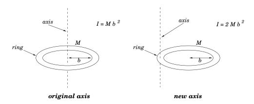
Figure 78: An application of the parallel axis theorem.
