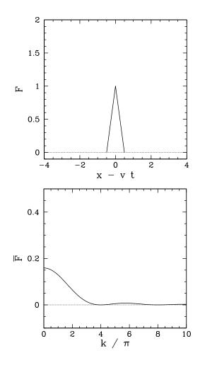
Figure 112: A propagating wave-pulse, F(x - v t), and its associated Fourier spectrum,  $\overline{F}(k)$ .
