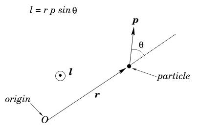
Figure 85: Angular momentum of a point particle about the origin.
