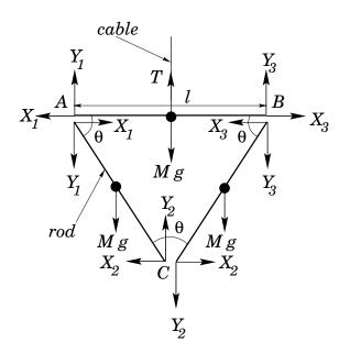
Figure 94: Three identical jointed rods.
