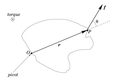
Figure 81: Torque about a fixed point.
