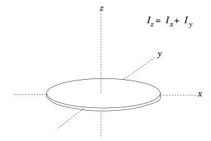
Figure 76: The perpendicular axis theorem.
