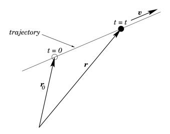
Figure 14: Motion with constant velocity
