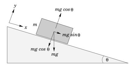
Figure 29: Block sliding down an incline
