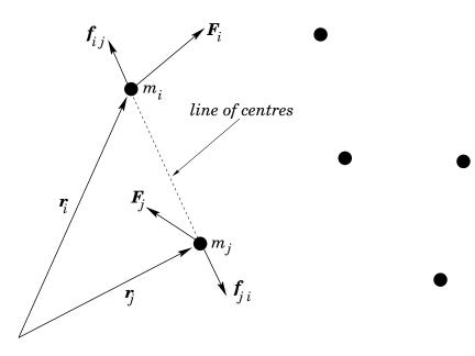
Figure 87: A multi-component system with central internal forces.
