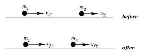
Figure 54: A collision in 1-dimension.
