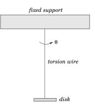
Figure 96: A torsion pendulum.
