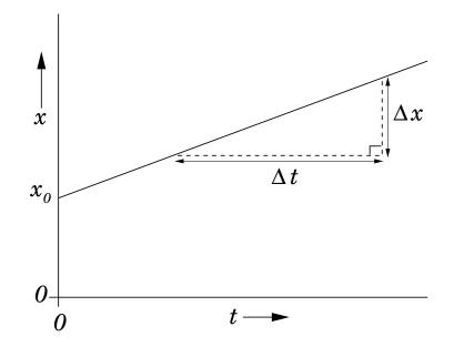
Figure 6: Graph of displacement versus time for a body moving with constant velocity
